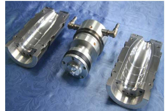
Quick change Blowing mold for Krones blower
