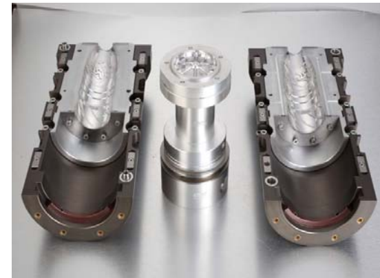
The blowing mold is settled on the mold shell
