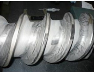
New wear-resistant alloy screw
